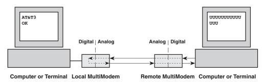
Figure C-3. Local digital loopback test.
